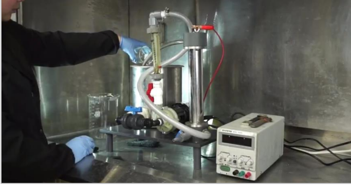
FIGURE 16 - EXTRACTION OF GOLD FROM SOLUTION USING A LAB SCALE EMEW® CELL
